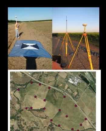
Survey-grade GPS and a significant number of ground control points for accurate image stitching
