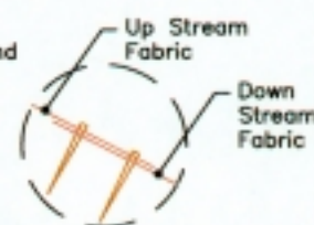
Key trench detail 2: Fabric-edge joints
