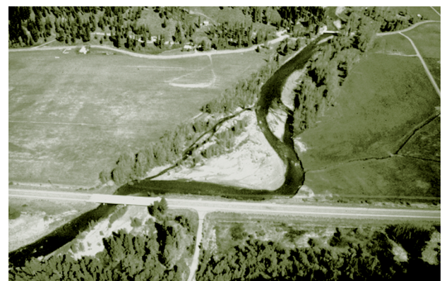
Figure 3-13. Meander extension and compression, Teanaway River, Washington State.
