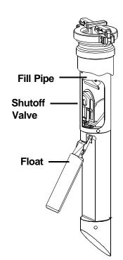
Some automatic shutoff devices work in two stages. The first stage drastically reduces the flow of product to alert the driver that the tank is nearly full. The driver can then close the delivery valve and still have room in the tank for the product left in the delivery hose.
