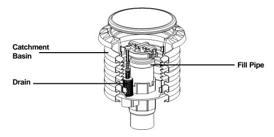
You should try to keep water out of catchment basins. Some catchment basins can collect enough water and sediment, along with spilled product, to make draining this mixture into the tank unwise. If this happens, you may pump out the catchment basin and dispose of the liquid properly. If the liquid contains fuel or chemicals, it could be considered a hazardous waste. Contact your state agency responsible for hazardous waste for information on testing and handling requirements.
