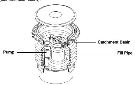
To protect against spills, the basin should be large enough to contain what may spill when the delivery hose is uncoupled from the fill pipe. Basins range in size from those capable of holding only a few gallons to those that are much larger-the larger the catchment basin, the more spill protection it provides.
