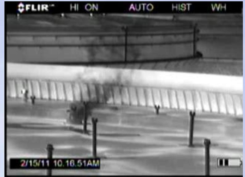
Storage vessel bleeder vents must be closed at all times unless the tank roof is being landed or floated off the leg supports
