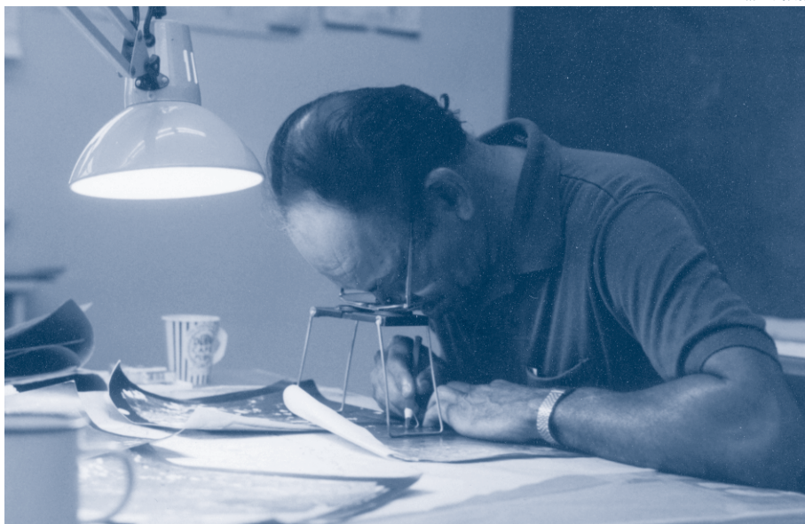
Figure 13. Aerial Photograph Interpreter Hugo Solis, of Panama's National Geographic Institute, studies photographs of the Darién using a pocket stereoscope.
